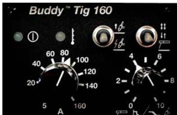
The control panel on the Buddy™ Tig 160 features one adjustment knob to set the weld current and one to set the slope down time in TIG mode or the arc force in MMA mode.
